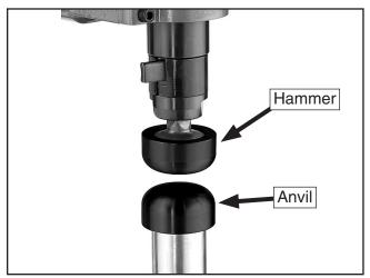
Figure 4. Planishing hammer and anvil.
